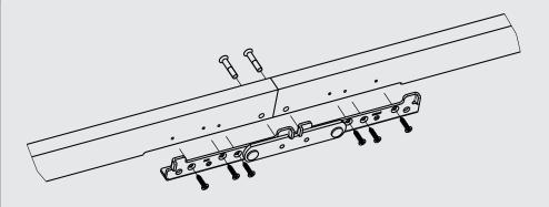
We recommend fixing each folding hinge on the outer rail (subject to a thickness of 20 mm) by means of 3 wood screws (M4.5 x 20 mm) and additionally by 2 countersunk screws M6x30 mm.
